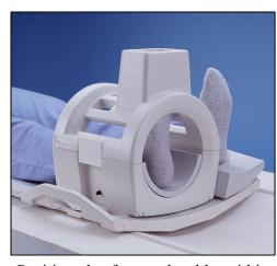
Position the foot and ankle within the coil. (Note: Ankle/foot pads not shown for detail.)
